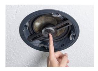
The two-piece baffle/speaker module assembly allows Partners to easily remove the speaker while leaving the cradle and grille in the ceiling or wall – preventing the speaker from being stolen or damaged during the construction process and allowing for HVAC pressure testing for certification of occupancy.
